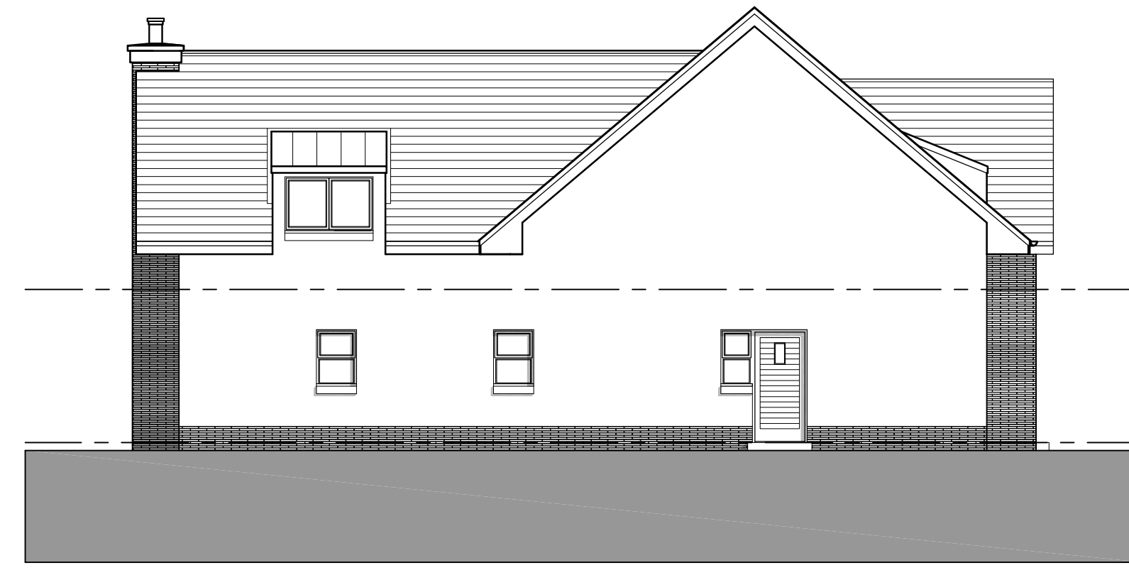
SIDE EAST ELEVATION, 1:100
